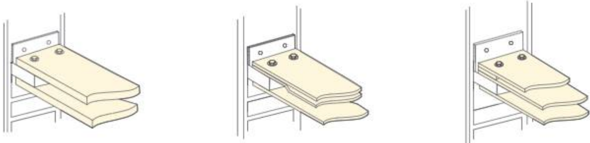
Figure 6.6-2 Recommended installation diagram of busbar
