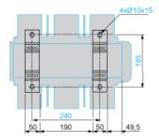
NOTE: X1 (mm) = Minimum electrical clearance according to operating voltage and breaking capacity.
