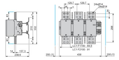
(1) Minimum distance required for coil removal.
