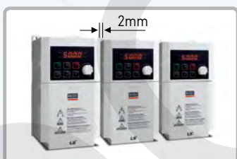
Side-by-side Installation (2mm between drives)
